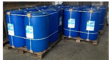
Drums strapped to pallet
