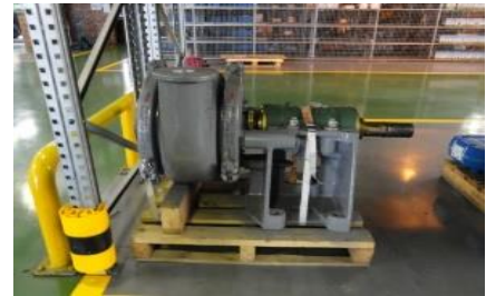
Material with balancing pin bolted to pallet
