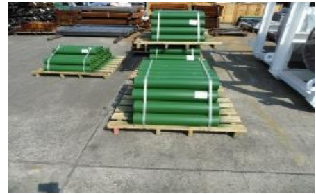
Material configuration of two ends strapped to pallet
